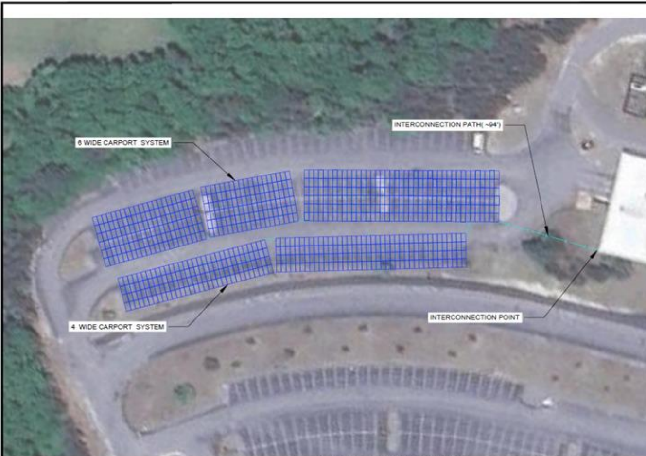
PROPOSED PV SOLAR ARRAY LAYOUT 1-50'
